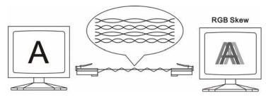
Recommend to use following cabling way to reduce skew status, to add special made "skew immunized adaptor", 2 pieces included at the package.
