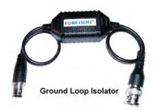
The GB001 Video Ground Loop Isolator is passive devices which reduce Ground Loop Interference with CCTV signals and can easily install in a new or added to existing systems. It is useful where a video signal is transmitted via cable between points with different ground potentials, Differences in ground potentials are typically caused by unbalanced power line loads.
